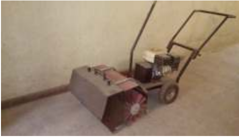
Fig. 14. Walk behind street sweeper mounted on wheels powered by gasoline engine
