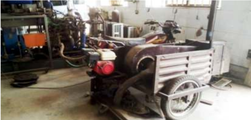
Fig. 13. Sucker type street sweeper mounted on wheels attached to a motor cycle.
